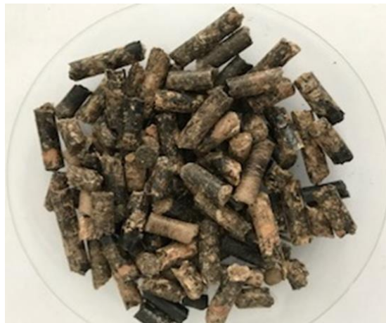
Figure 2. Pellets from sewage sludge + beech sawdust ESS SS + BS (II)
