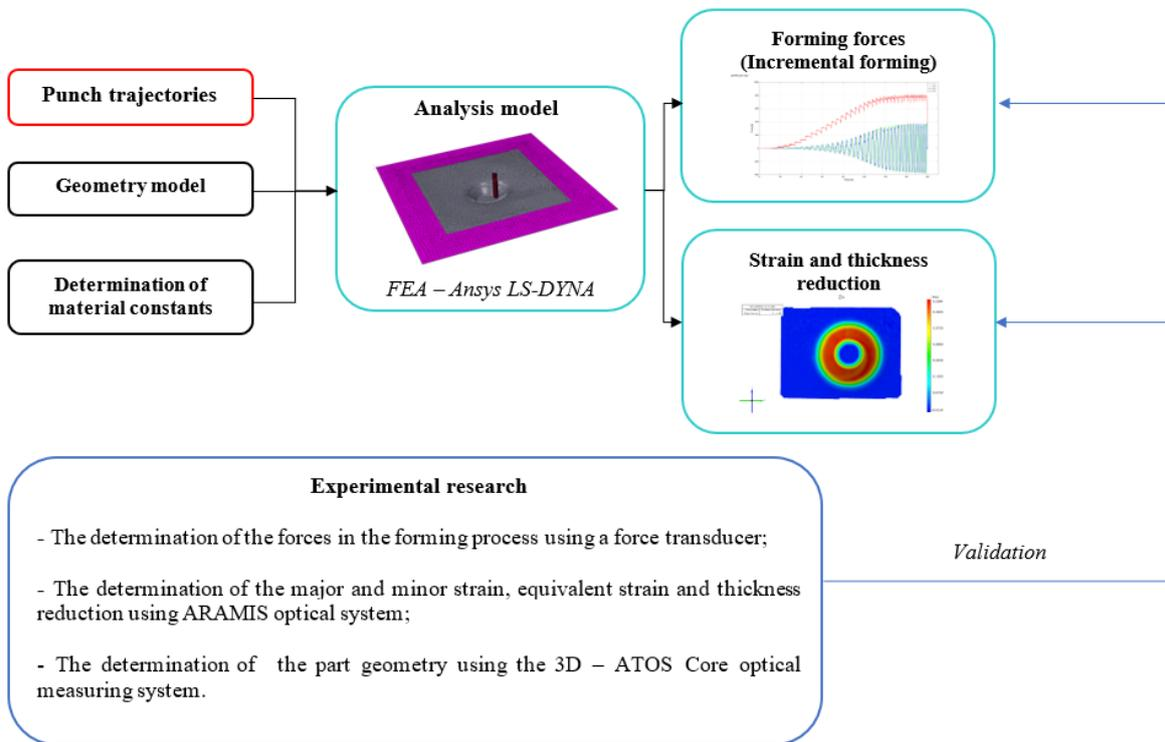
Fig. II: Validation block diagram of the analysis model using FEM.
