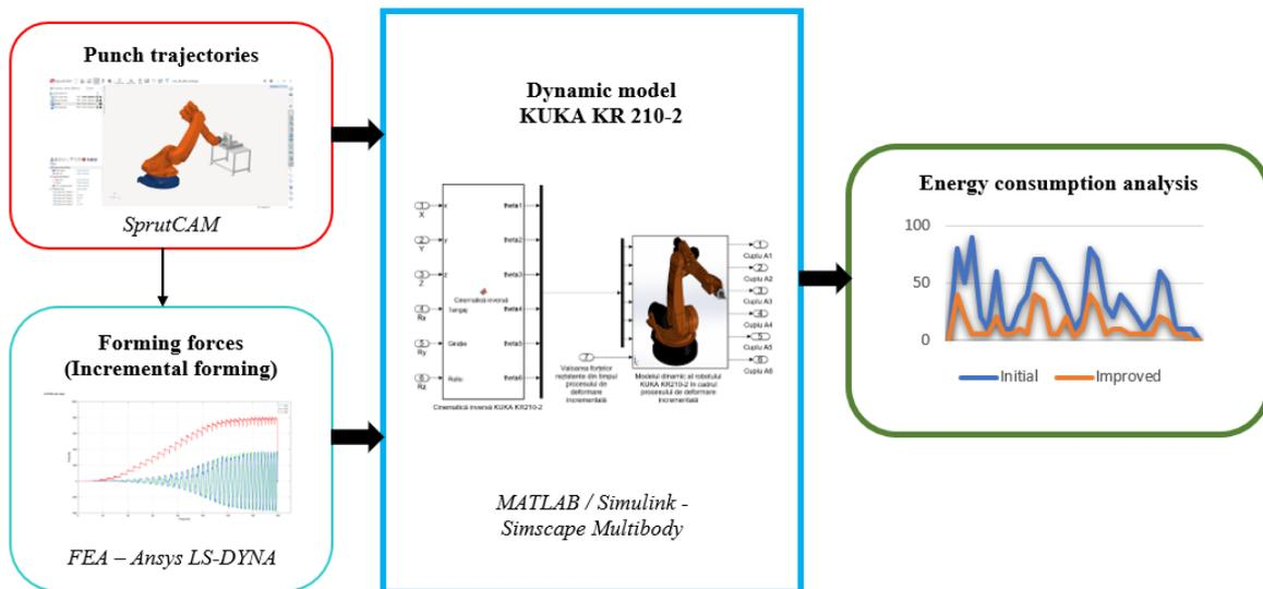
Fig. 1: Block diagram corresponding to the development of the algorithm for establishing energy consumption.
