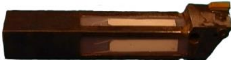
Figure 1.2. First attempt at an active tool support solution using the technique piezo - ceramic for vibration attenuation [56]
