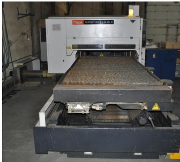
Fig. 5.1: Laser cutting machine with numerical control, brand MAZAK ST-X48 Mk II
