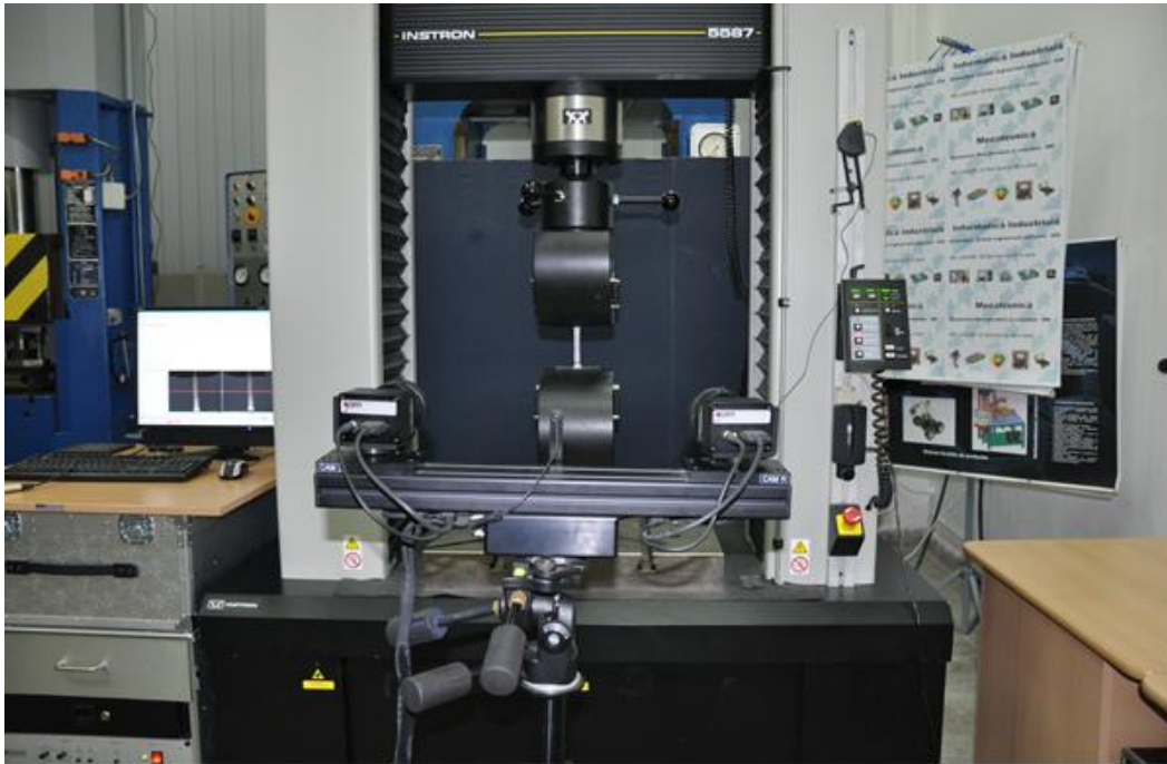
Figure 5.1. Machine to testing tensile uniaxial Instron 5587
