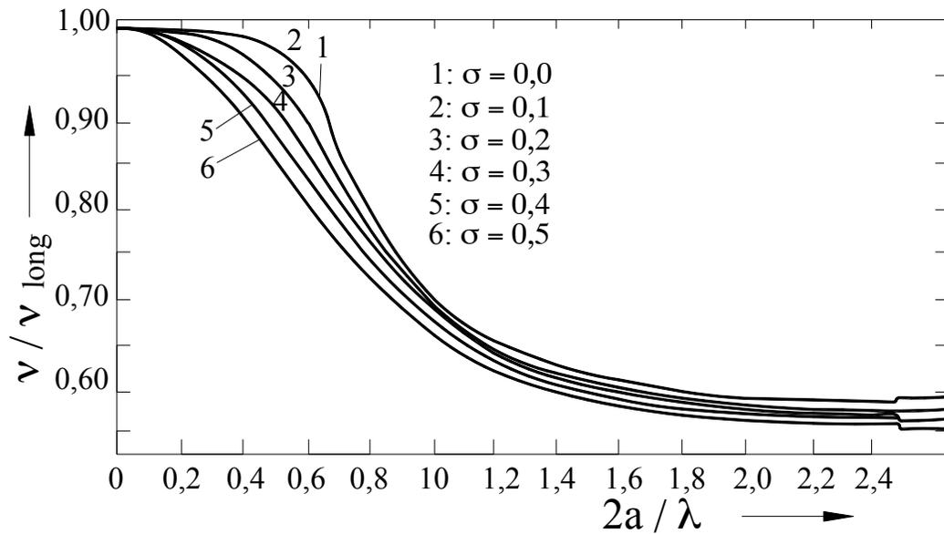
Fig. 4.18. The dependency of the  $v/v_{long}$  coefficient, of  $2a/l$  size, for different values of the Poisson's ratio.
