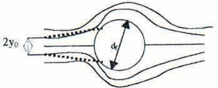
Fig. 2.1 The image of the hydro-dynamic spectrum at small Reynolds numbers at the movement around a cylinder (a fiber)
