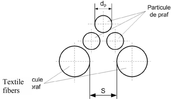
Fig. 2.6. Placement of textile material fibers and dust particles inside a filter;  $d_p$  diameter of solid particles;  $s$ -distance between two textile fibers
