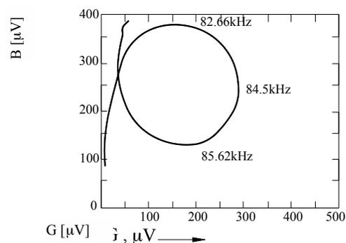
Fig. 4.14 Admission diagram of a piezoceramic complex transmitter  $G = f(B)$ .
