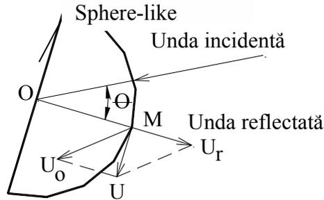
Fig. 3.7. Angular allocation of the particle's speeds at the diagonal incidence of an ultrasound beam on a circular obstacle
