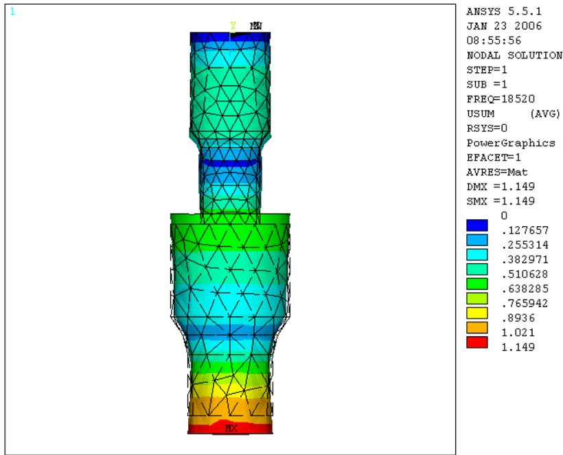
Fig. 5.22. The vertical representation of the deformed/non-deformed state of the intermediary element – concentrator ensemble at 18520 Hz.
