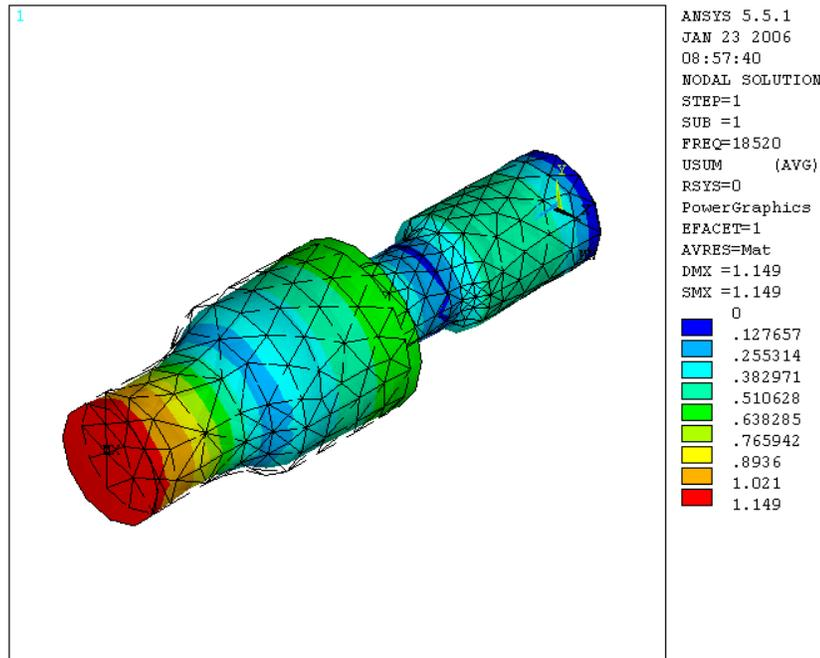
Fig. 5.21. The isometric representation of the deformed/non-deformed state of the intermediary element – concentrator ensemble at 18520 Hz.
