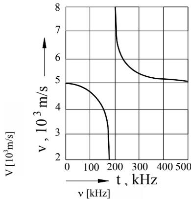
Fig. 4.17. The geometrical dispersion of longitudinal waves in a nickel rod of 100 mm length, an exterior diameter of 8,6 mm and an interior diameter of 8,3 mm.
