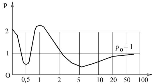
Fig. 3.10. Variation of the ultrasound pressure in the shadow area of a normal circular obstacle on the beam's direction
