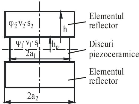
Fig.4.21. Symmetrical complex piezoceramic transmitter.
