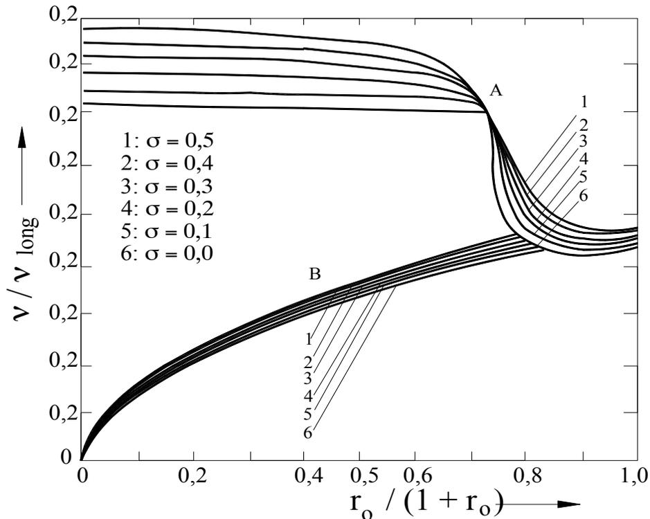
Fig. 4.19. The theoretical dispersion curves of longitudinal waves A and shear waves B
