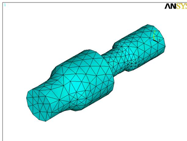
Fig. 5.20. Finite element meshing of the volume of the intermediary element – concentrator ensemble.
