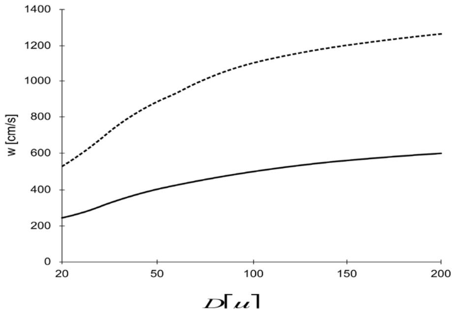
Fig.2.2 The entrainment and floating beginning speed of the dust particles
