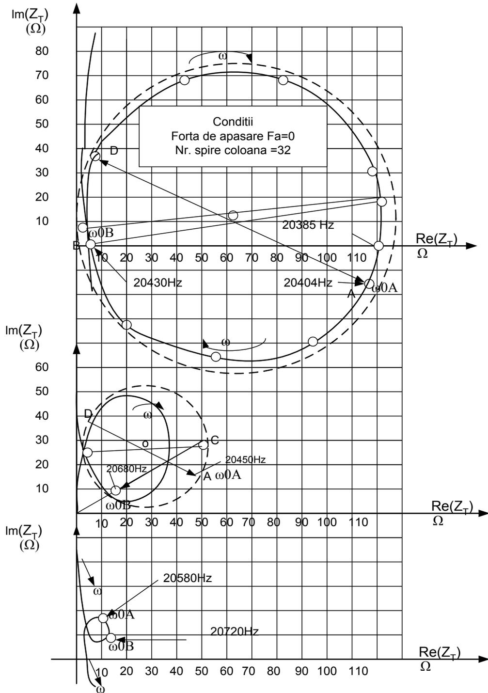
Fig. 4.20. The variation mode of „ $Z_T$ ” impedance for the concentrator transducer ensemble of the ultra-acoustic system used in experiments.
