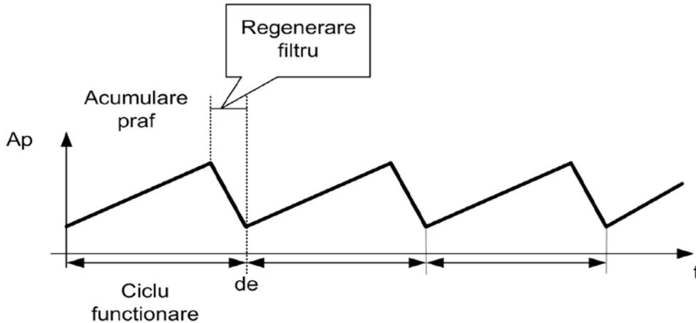
Fig. 2.7 The functioning cycles of the filtering device
