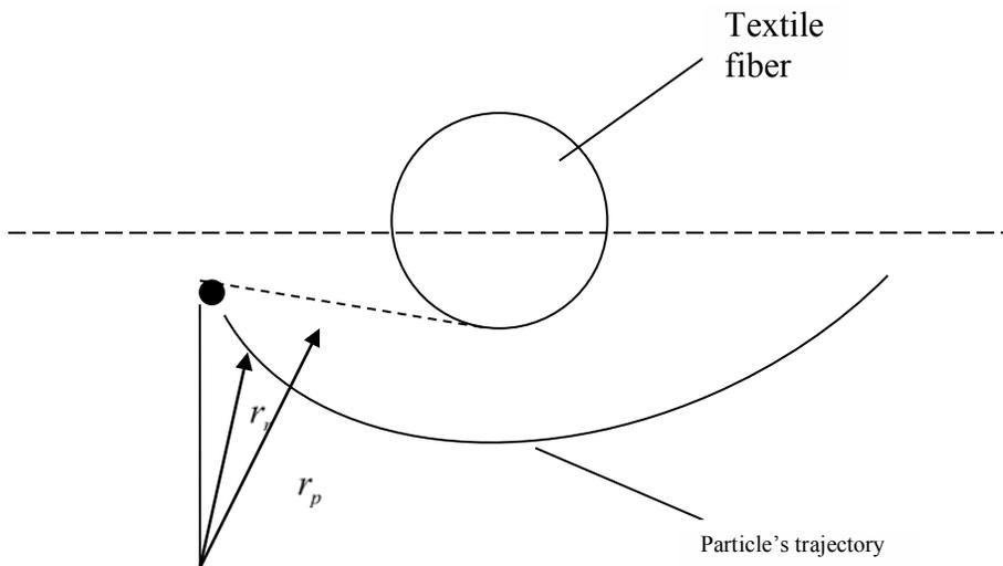
Fig. 2.2 Movement of the fluid particles around a textile material fiber
