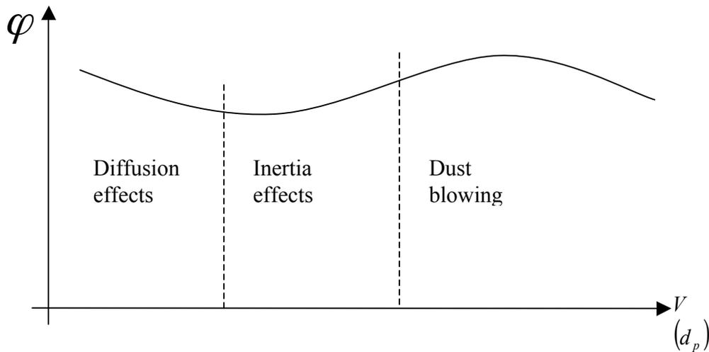
Fig. 2.8 Functioning cycles of the filtering device
