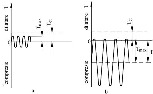
Fig.4.12. The influence of mechanical polarization  $T_0$  over the maximum value of the mechanical tension  $T_{max}$ , which can be applied to the complex transducer during operation:
