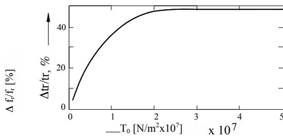
Fig. 4.13. The influence of the mechanical polarization tension  $T_0$  over the resonance frequency of the transmitter
