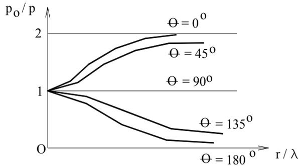
Fig. 3.8. The variation curves of the  $p_o / p$  ratio according to  $r / \lambda$ .
