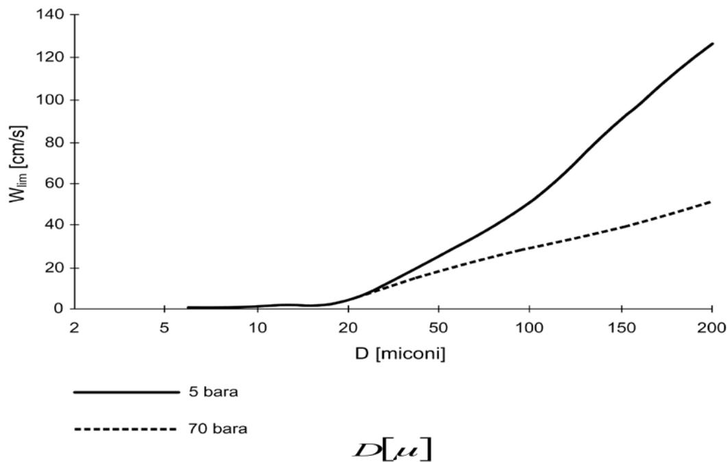
Fig.2.1 The minimum falling speed of dust particles
