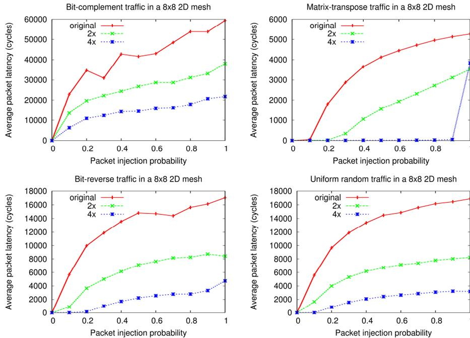
**Fig. 7 The average packet latency on a 8x8 Irvine NoC architecture, while the speed with which data flits advance in the network varies for 4 different communication patterns**
