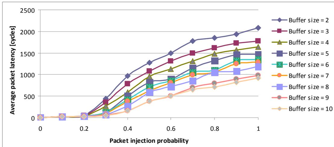
Fig. 8 The average packet latency on a hypercube NoC architecture, while the size of the input buffers varies uniformly
