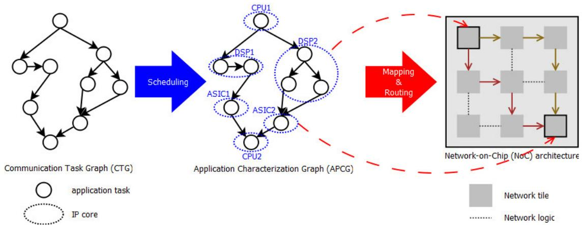
**Fig. 4 The scheduling, application mapping and routing problems**
