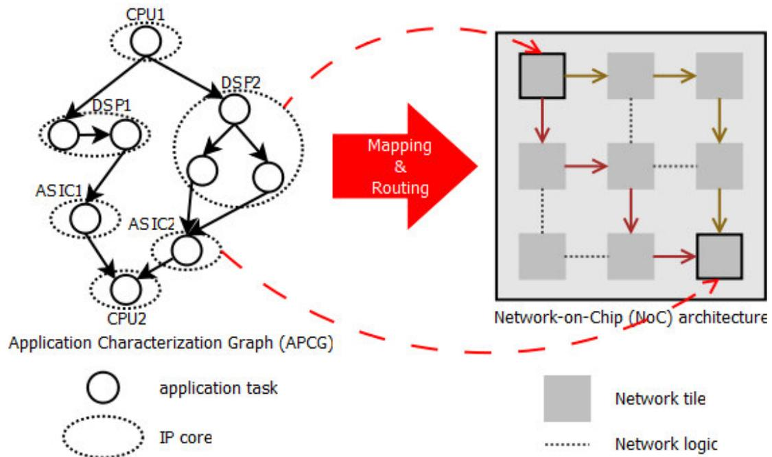
Fig. 3 The application mapping and routing problems
