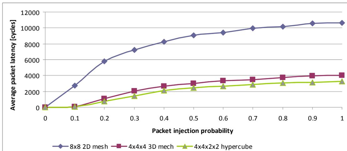
Fig. 9 Average packet latency on 64 node mesh NoCs, with 2, 3 and respectively 4 dimensions
