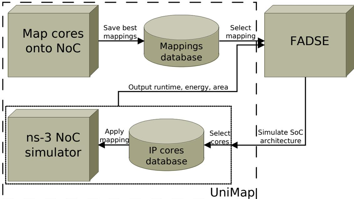
Fig. 26 Application driven DSE workflow for SoC designs
