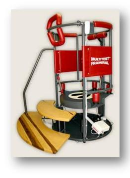
computerized device built from a platform fitted with movement sensors that can register the variations of the gravitational line of the body.
