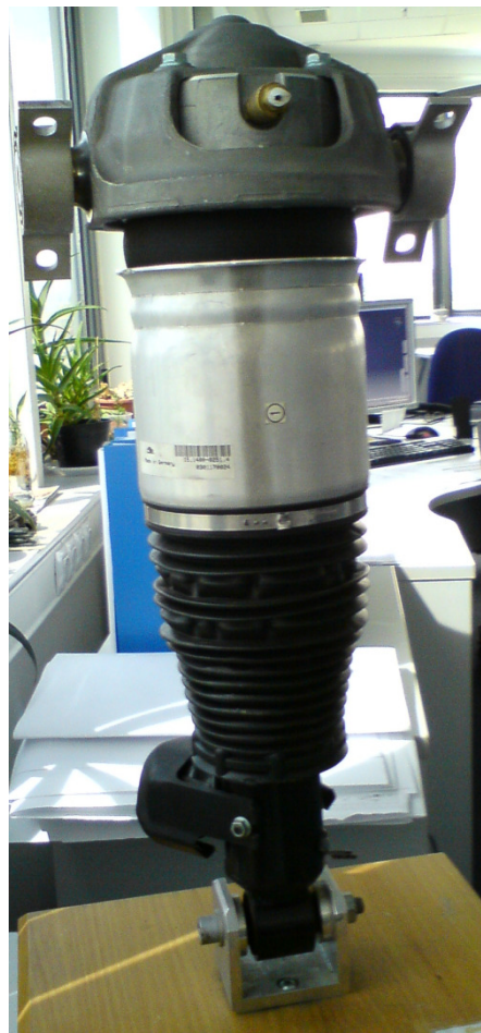
Figure 2.3.1. Continental AG developed pneumatic suspension (VW Touareg / Porsche Cayenne)
